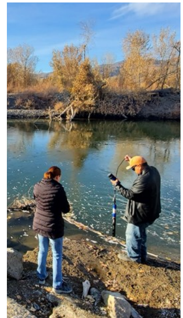
WQ Team members taking field measurements using the YSI EXO 1 sonde along the Truckee River
